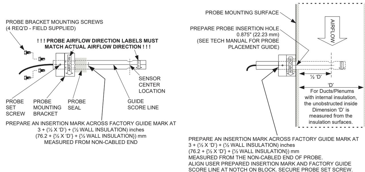
**Figure 6. GF-A2100 Single Probe Insertion Mount Detail for Economizer Hood and Duct Applications**
