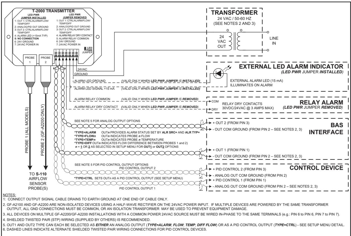
Figure 10. GF-A2100/GF-A2200 Wiring Diagram Detail
