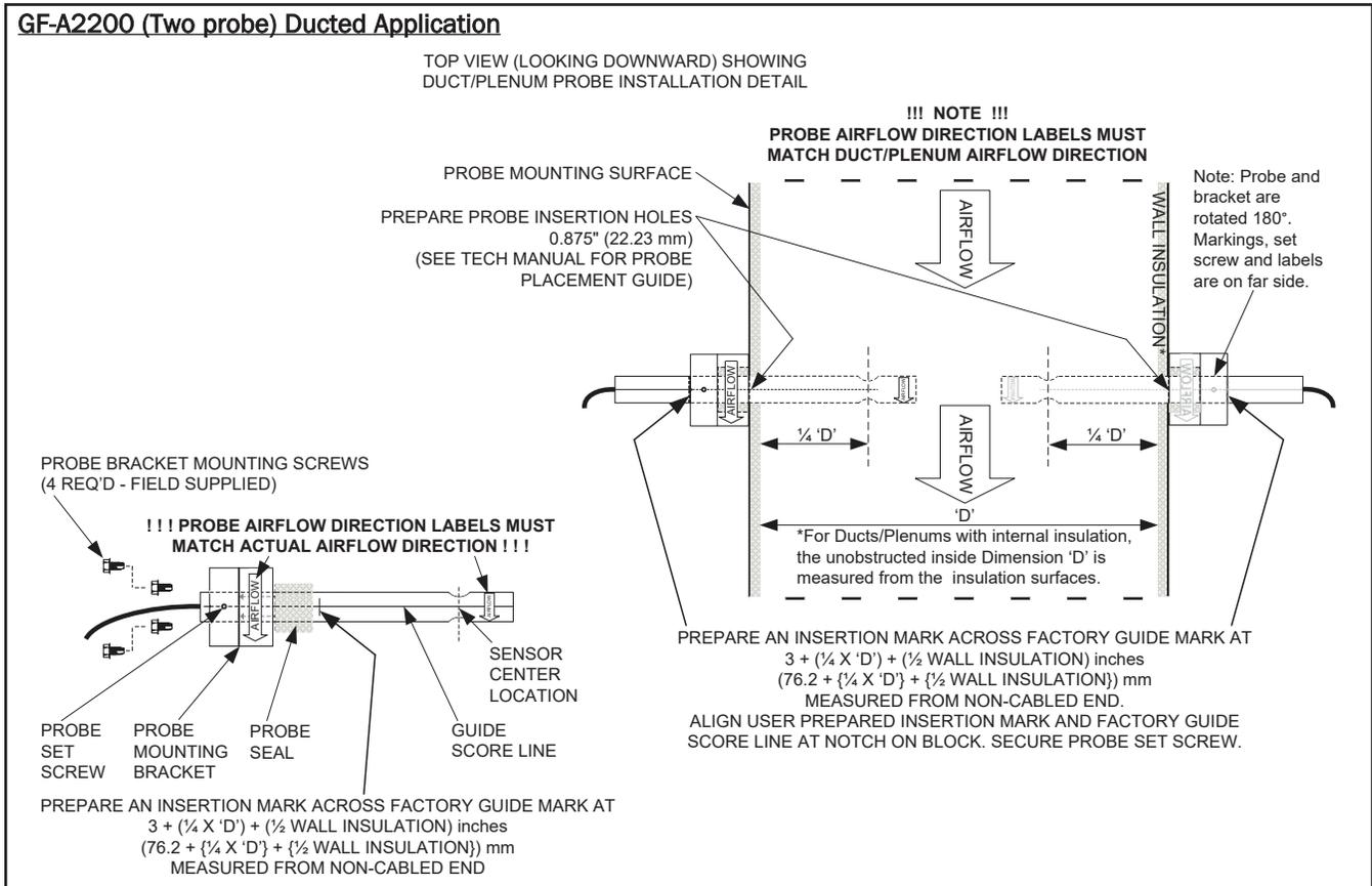
Figure 7. GF-A2200 Two Probe Insertion Mount Detail for Economizer Hood and Duct Applications
