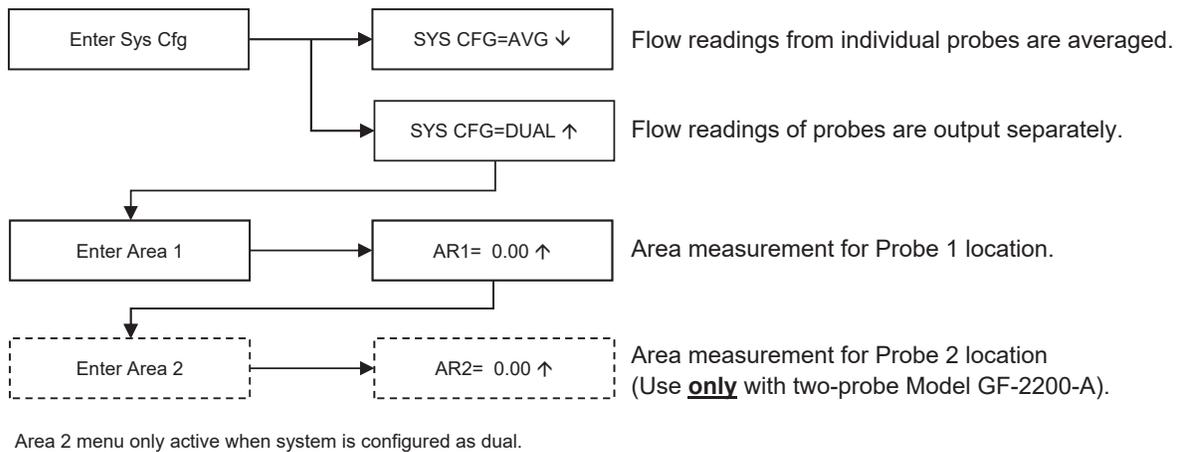
**Figure 11. Transmitter Start Up Menu**
