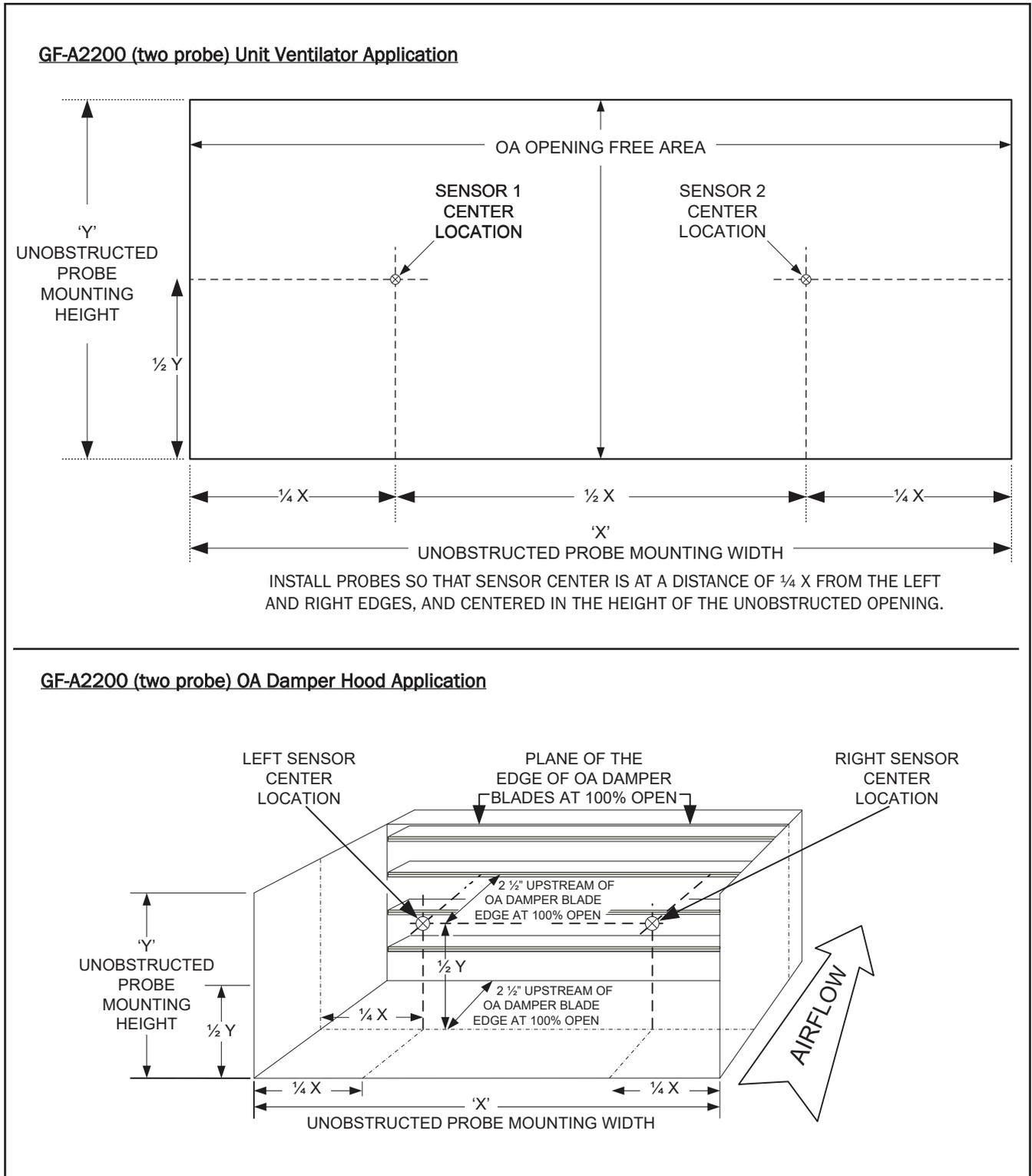
**Figure 4. Universal Mount Probe Detail for Unit Ventilator and OA Damper Hood Applications**
