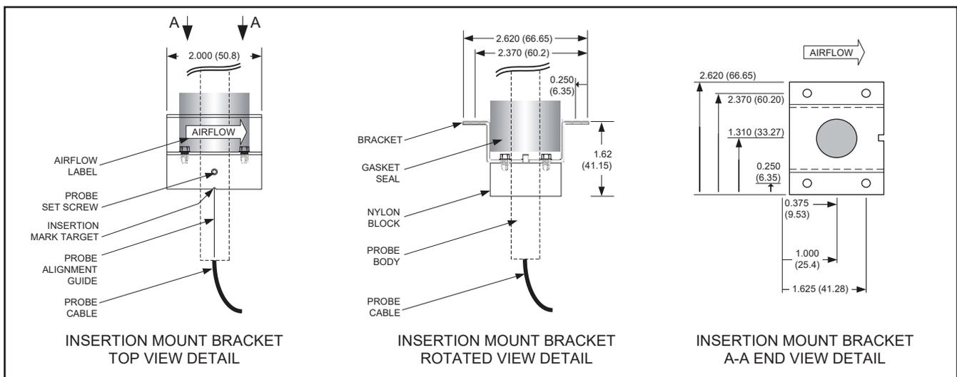
**Figure 5. Insertion Mount Probe and Bracket Mechanical Detail**
