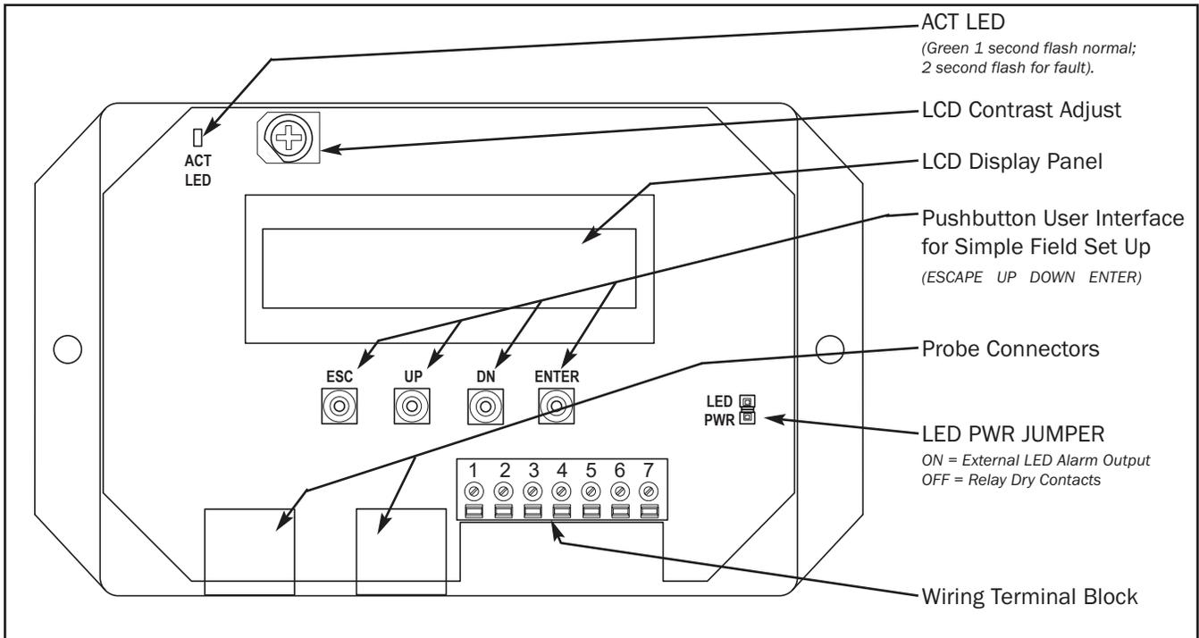
Figure 9. GF-A2100/GF-A2200 Main Circuit Board Detail
