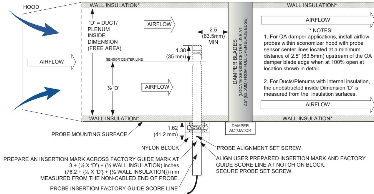
**GF-A2100 (Single probe) Ducted Application**
