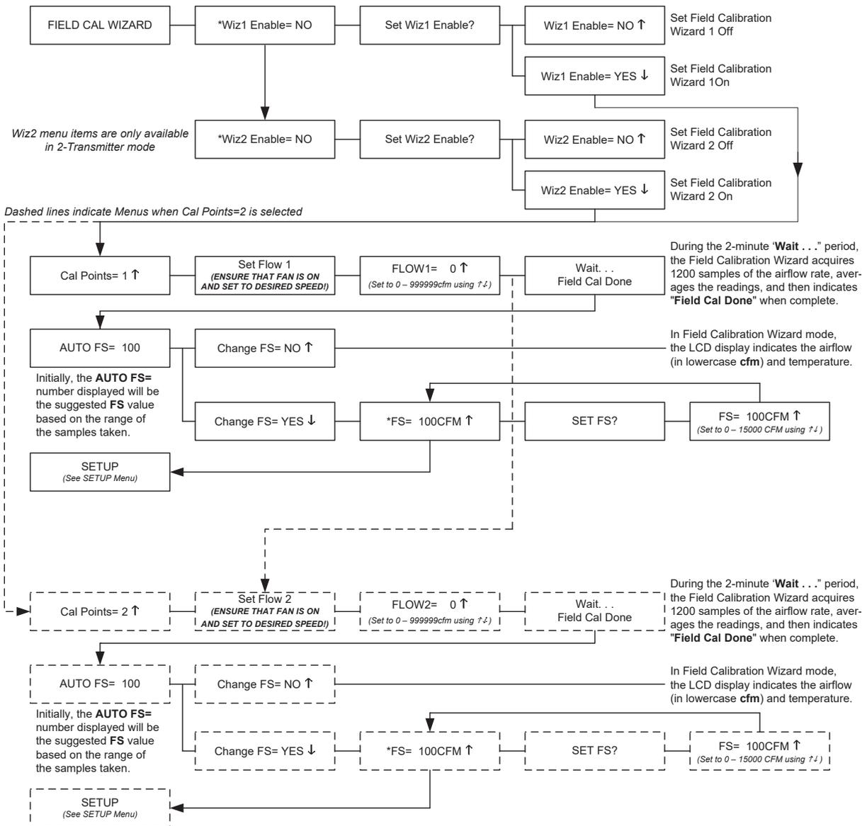
Figure 16. Field Calibration Wizard Menu (all System of Units)
