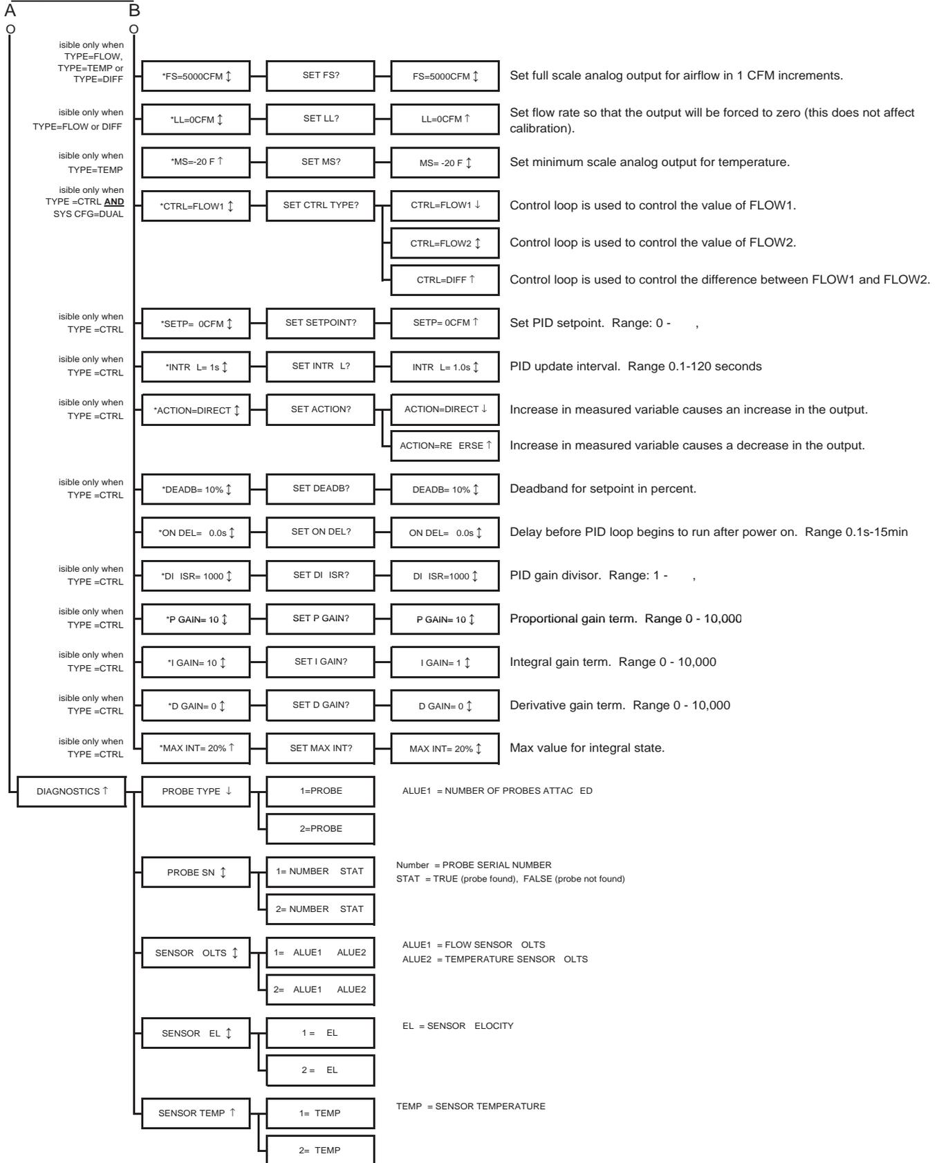
Figure 15. (part 3 of 3) GF-A2100/GF-A2200 Setup Menu Option ("IP SYS")
